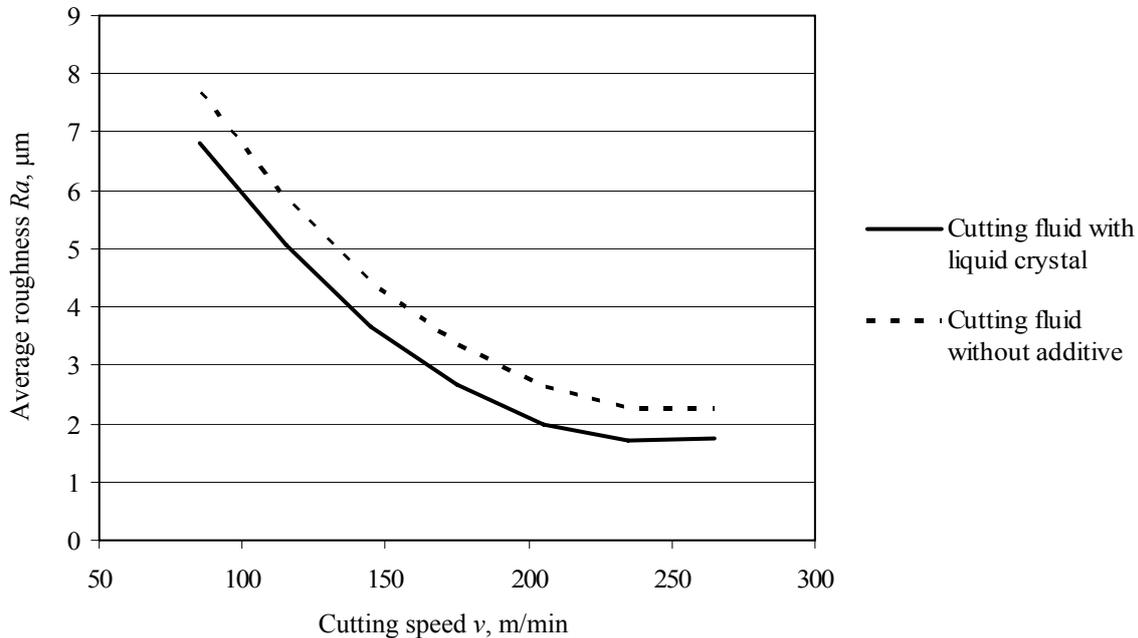
Fig. 3 Average roughness  $Ra$  of turned surface as the function of cutting speed  $v$  and composition of the cutting fluid
