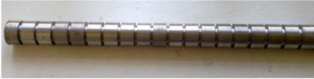
Fig. 2 Steel bar divided into the sections
