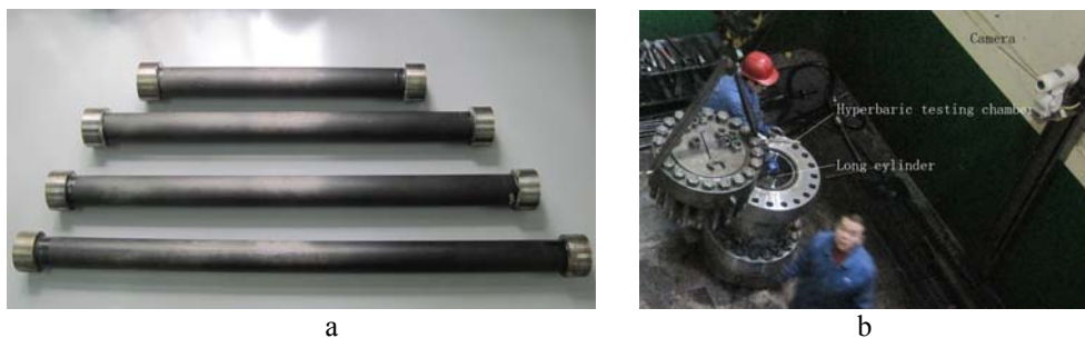
Fig. 3 a - composite long cylinder; b - hyperbaric testing chamber for external hydrostatic pressure test
