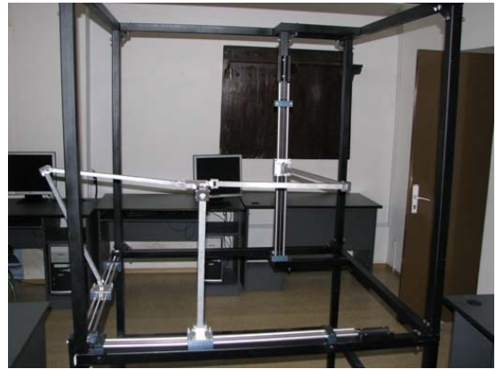
Fig. 2 ISOGLIDE3 parallel robot realized at Mechatronics Department
