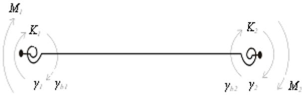
Fig. 4 Beam-column element with flexible connections
